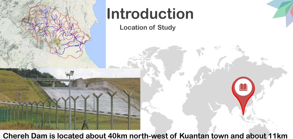
Chereh Dam is located about 40km north-west of Kuantan town and about 11km north of Lembing River. The main features are: an earth fill embankment dam of 4 8m high with a 50m width un-gated chute spillway. Surface are is 54km<sup>2</sup> and volume is 250 x 10<sup>6</sup> m<sup>3</sup>
